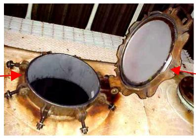
INERTEX® Inermet RRTC Gasket Dome Lid Design (Type DL)
